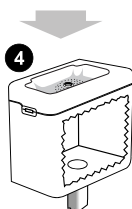
CISTERN EMPTY READY FOR NEXT USE
