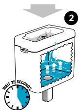
CISTERN FILLS WITH WATER
